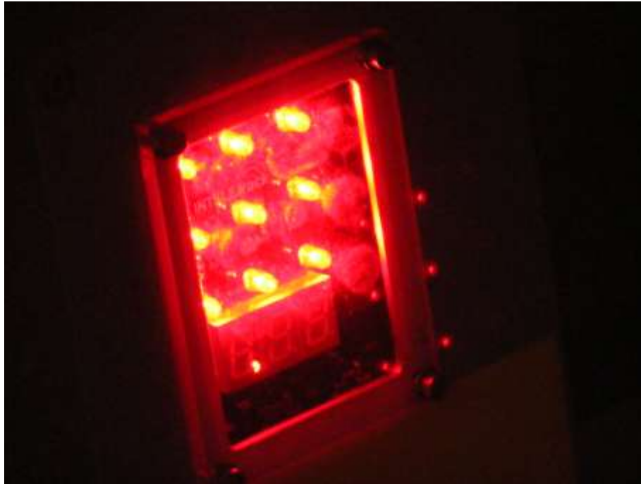
Figure 29: The flasher circuit actually detecting bad light and flashing.
