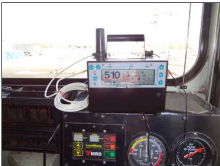
Figure 4: The Inteltrack 'One Touch' in a portable configuration inside a locomotive. This is usually a configuration used for testing and for use in some specified areas. The CU will usually be installed into a designated compartment within the locomotive.
