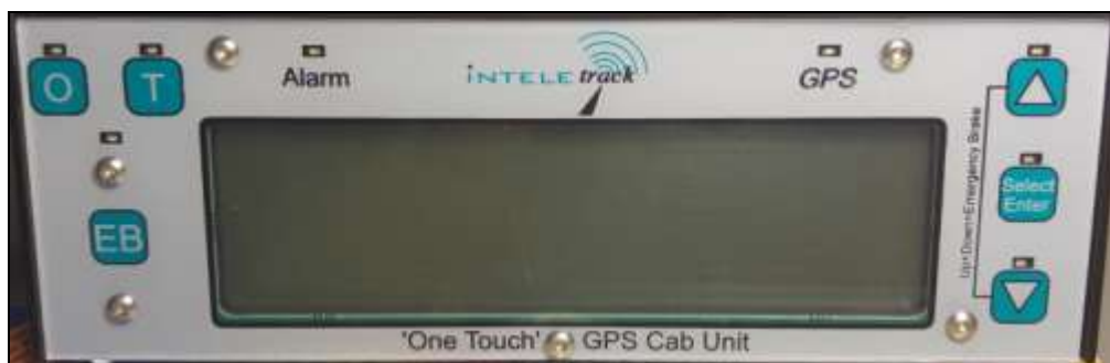
Figure 3: The front panel of the 'One Touch' HoT monitor; also called the cab unit. The capacitive touch buttons, indicator LEDs and graphic display can be seen.
