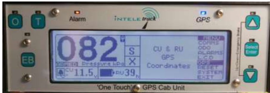
Figure 33: Getting to GPS information from the operational menu.
