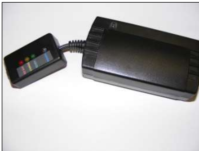
Figure 31: The rear unit charger with charge indicator module attached.
