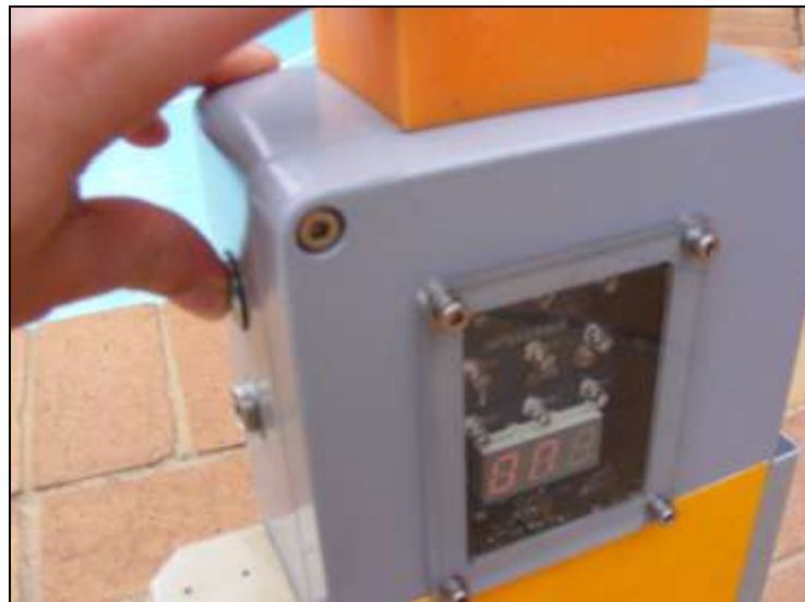
Figure 16: By pressing and holding the push-button on the RU, the unit is switched on. Release button when "ON" is displayed on the 7-segment display.
