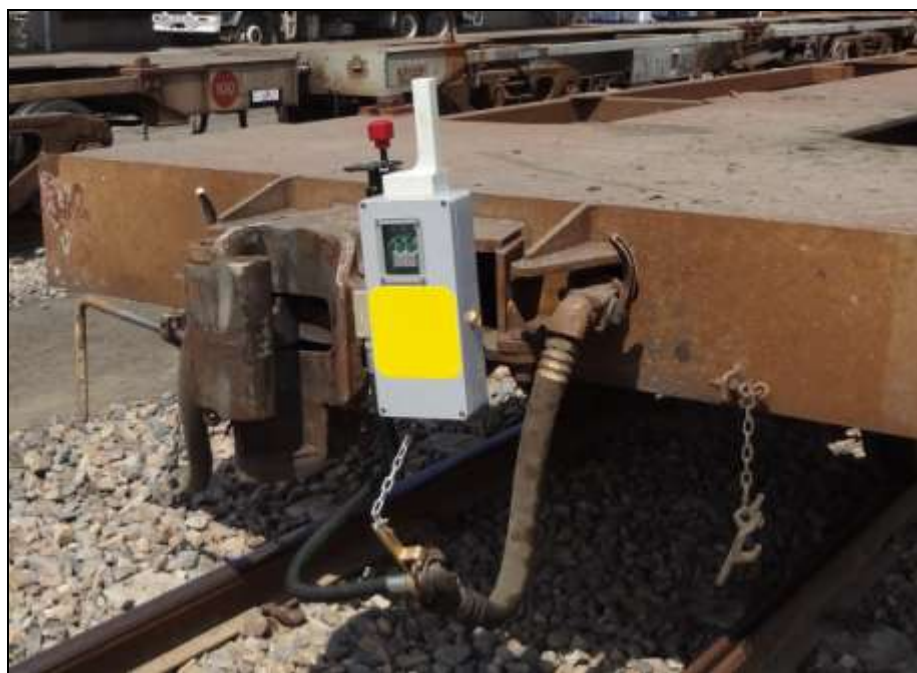
Figure 2: The Inteltrack GPS3 mounted onto a rear buffer.
