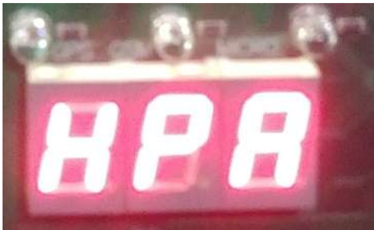
Figure 22: Second menu shows pressure units.
