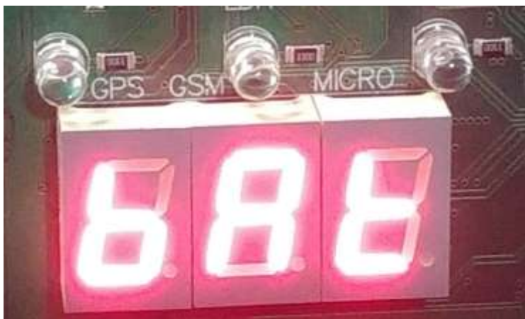
Figure 24: Fourth menu shows 'bAt', indicating that the voltage displayed is that of the RU power source.
