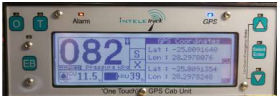
Figure 34: The GPS information displayed with other information. Here it is clear to see that both CU and RU have valid GPS coordinates.
