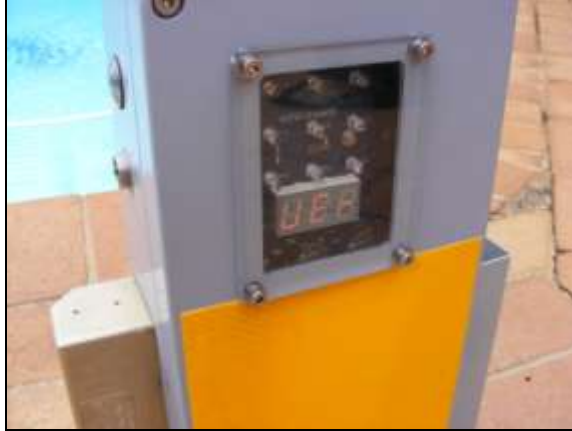
Figure 17: After the RU has been switched on, “VER” is displayed on the 7-segment display. The version number of the firmware used is displayed next.
