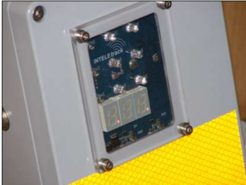
Figure 27: The flasher circuit actually detecting bad light and flashing. The indicator dots indicate bad GPS signal and processor running.
