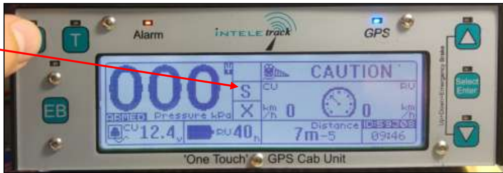
Figure 9: If the correct length has been saved, the driver may use the Point Clear function to see the distance to drive until the point has been cleared.
