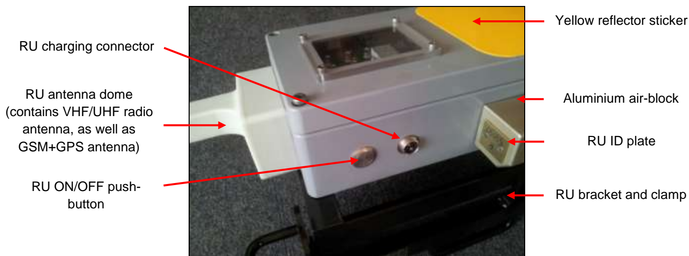
Figure 32: The rear unit parts.
