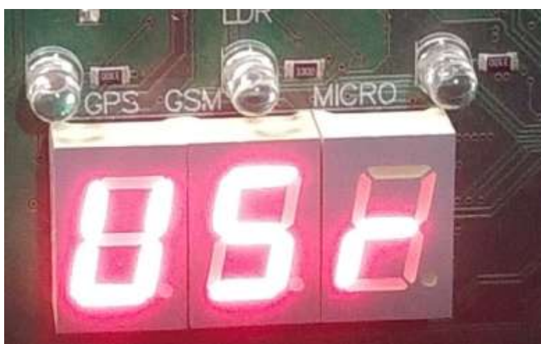
Figure 26: Sixth menu shows 'USr', indicating VSWR ratio.
