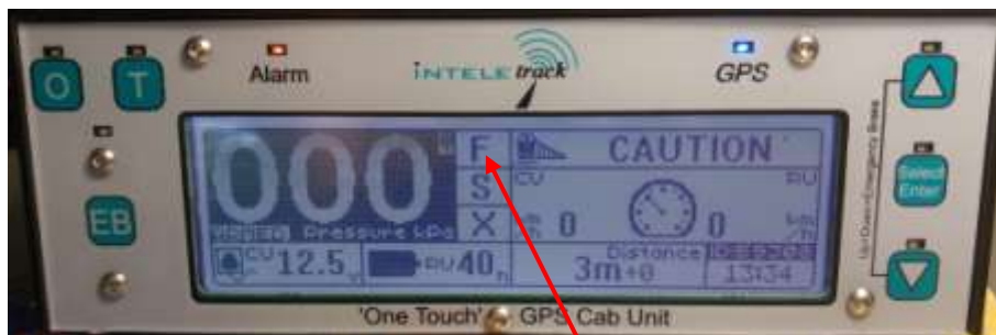
Figure 30: The flasher indicated on the CU.
