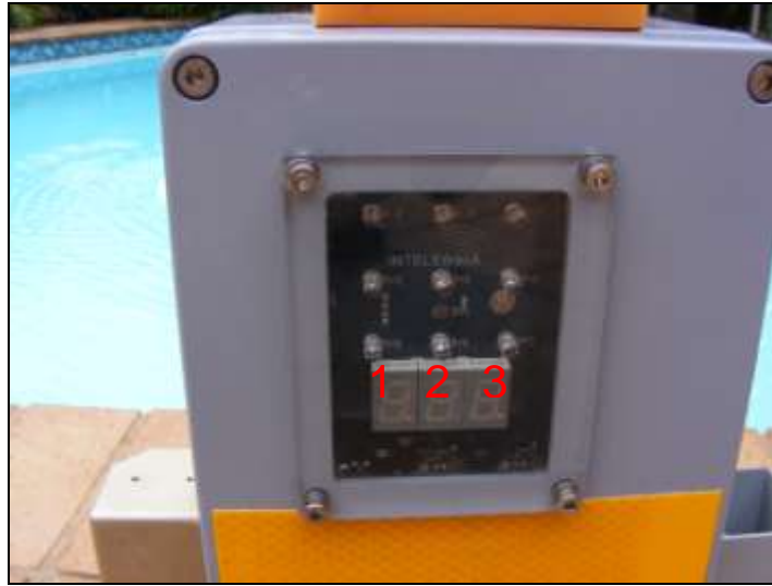
Figure 19: The dot indicators. GPS [1], GPRS acknowledged [2], processor running [3].
