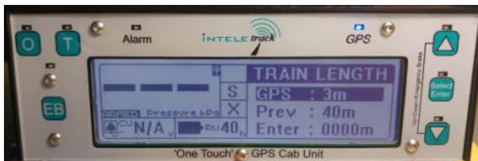
Figure 8: Train Length is important for the Point Clear function. Be sure to enter the correct train length as explained previously.
